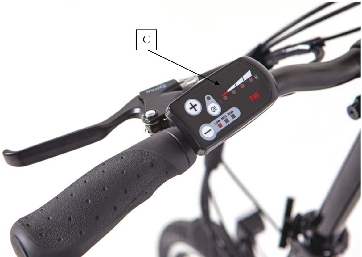
The red lights dots will indicate the battery level (you can check also by pressing the other indicator that is located on the battery). You can use the **Plus** and the **Minus** buttons to change the motor assist level. On low you get less power from the motor and you need to use more the pedals and on high you will get the full power from the electric bike. The light button is to turn on and off the front and the back light.
